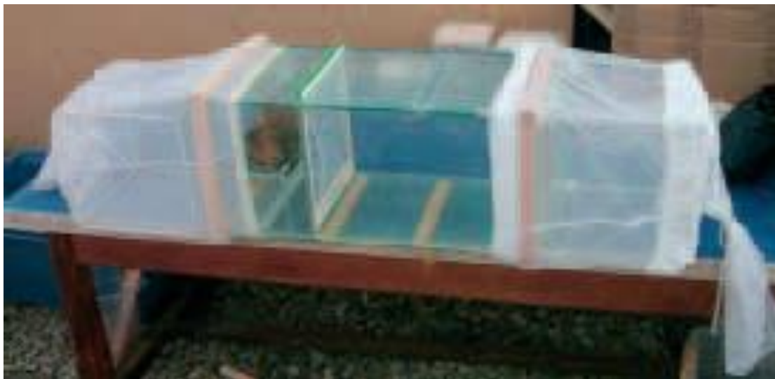
Fig 2. A tunnel made of glass for the study of the efficacy of insecticide-treated mosquito nets
